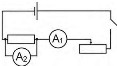
$$I_1 = I_2 + I_R; \frac{I_R}{I_2} = \frac{R_A}{R} \Rightarrow R_A = R \cdot \frac{I_1 - I_2}{I_2}$$
