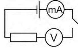
$$I_2 = I_R + I_V = \frac{U_2}{R} + \frac{U_2}{R_V} \quad (1) \quad R = \frac{U_1}{I_1} \quad (2) \quad I_3 \cdot R_V = U_3$$
