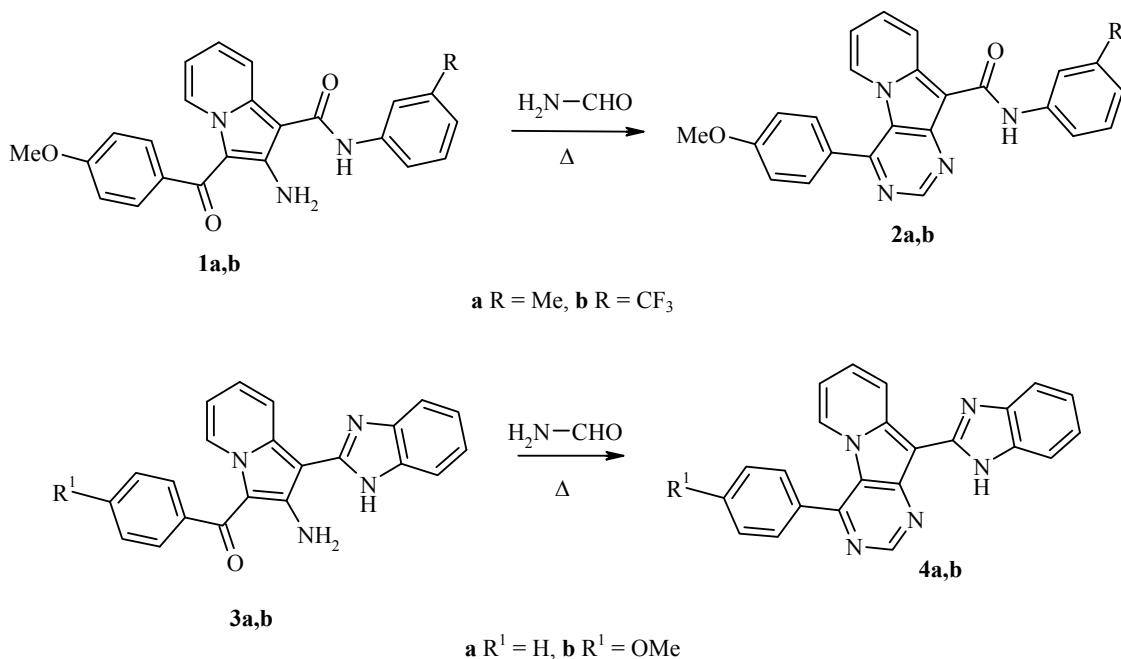
Only one of the two possible reaction routes is realized and this involves the amino and carbonyl groups. Hence, in the IR spectra of compounds **2** and **4**, signals for the amino and carbonyl groups are lost and signals appear which are typical of a secondary amide group and an imidazole NH group [2]. The mass spectrum of compound **2a** shows a signal of relative intensity 3.1% which corresponds to the molecular weight.
